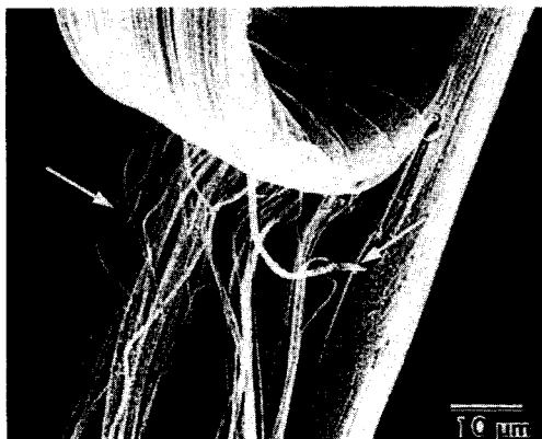
그림 9. Secondary electron image (SEI) of a polymer fiber (PET) prepared by the peelback method reveals the internal fibrillar texture (arrow).
