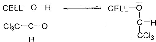
그림 4. Formation of acetal between cellulose hydroxyl group and chloral.
