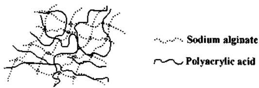
그림 3. Semi-interpenetrating polymer networks composed of sodium alginate and polyAAc.
