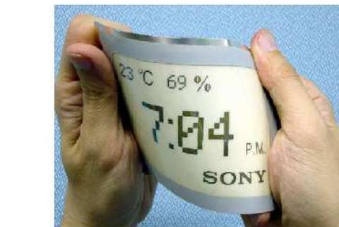
그림 5. Schematic representation of electrochemical deposition display system by SONY and its demonstration sample showing flexibility.
