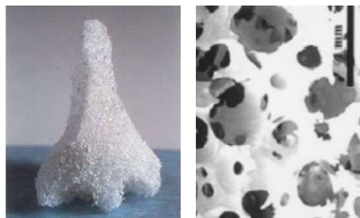
Human nose-like scaffold Pore morphology
