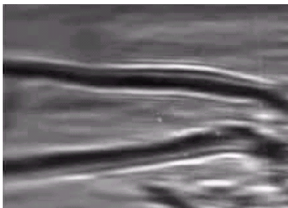
그림 5. Microscopic features put in evidence by coherence-related contrast in the radiograph of an ant leg. Diffraction-based interferences are clearly visible at the leg boundaries.
