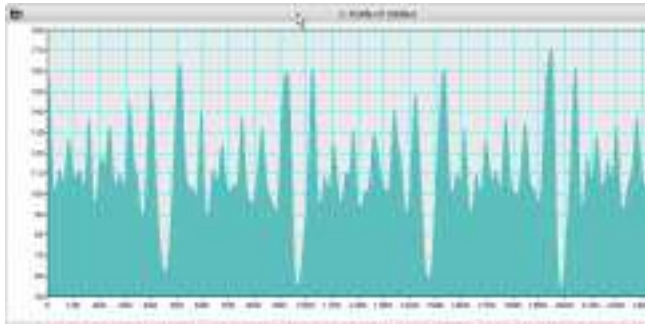
그림 22. Line profile for the lattice plane of \text{In}_2\text{O}_3(\text{ZnO})_5 with super-lattice structure.
