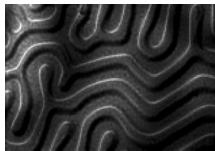
그림 31. Fresnel image of 200 nm wide domain walls in NdFeB. On the a domain strip, we can see the set of white and black lines. It gives a useful information, which we can define the spin direction in domain.
