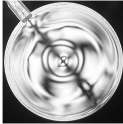
그림 14. Birefringence of lens made by injection compression molding.
