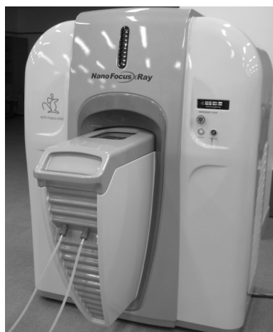
그림 3. Photographs of in-vivo micro-CT system. Note respiratory anesthesia tube for live animal study.
